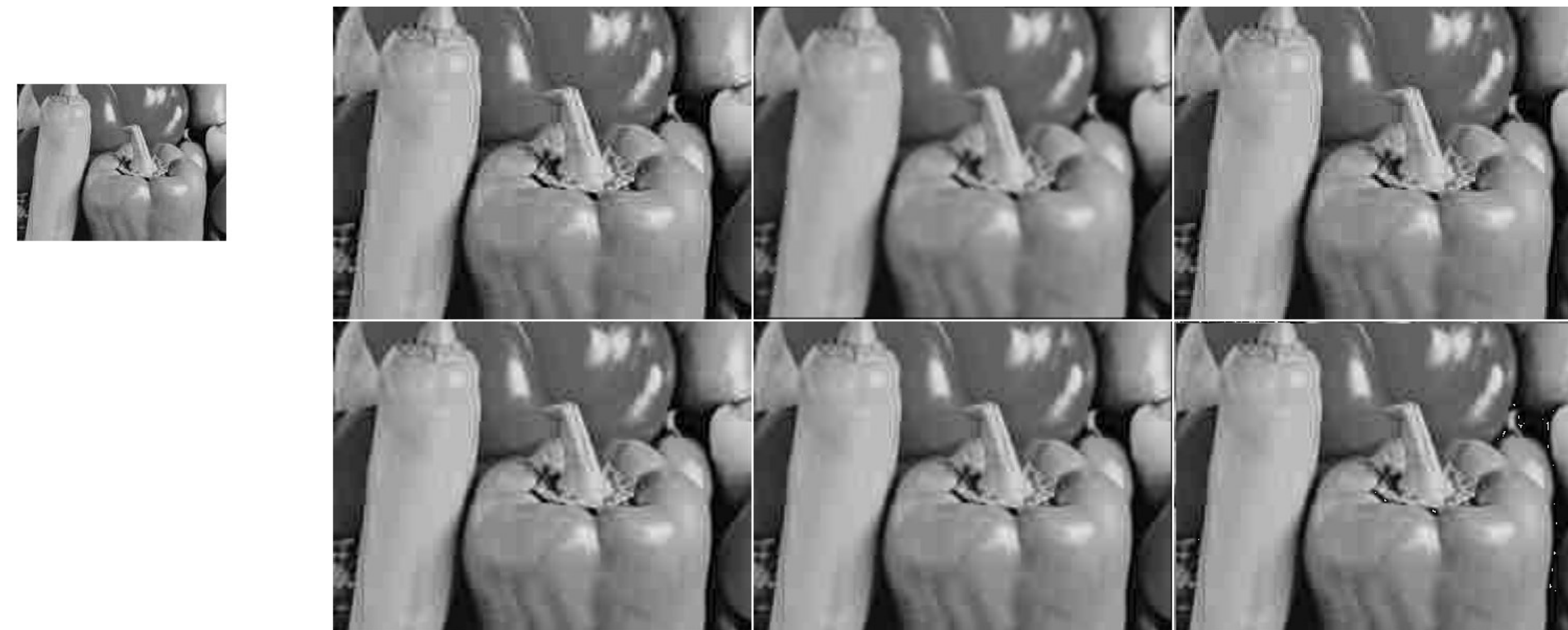
Figure 4: From top left to right image order: original low-resolution, super-resolution, super-resolution with JPEG enhancement, zero-order hold, lagrange, bilinear and bicubic.
